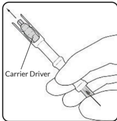
Push Carrier Driver forward like a syringe to attach and detach carrier from the QuickConnect Retainer.
