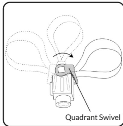
The Quadrant Swivel is used to swivel the band for use on any quadrant.
